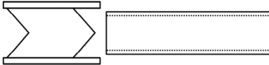
Figure 14.7. Removal of internal burrs from PVC pipe (right) with deburring tool (left).
