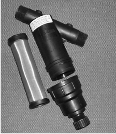
Figure 16.12. Course screen filters remove large particulate contaminants from the system.
