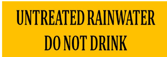
Figure 16.20. Label to be placed on piping and faucets to notify users of water quality.
