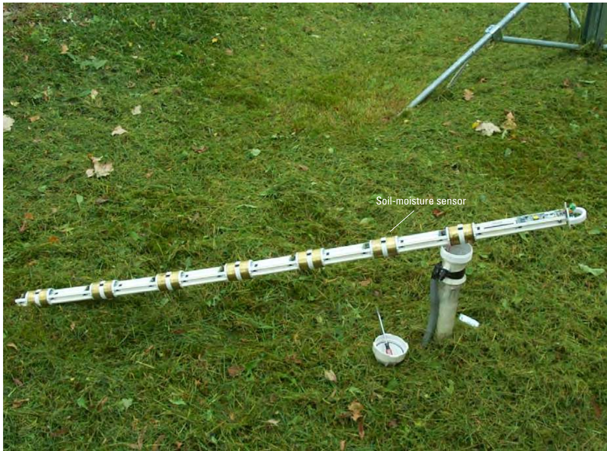
Figure 7. Soil-moisture sensors spaced at 20-centimeter intervals on soil probe. The soil probe is inserted vertically into the access tube.
